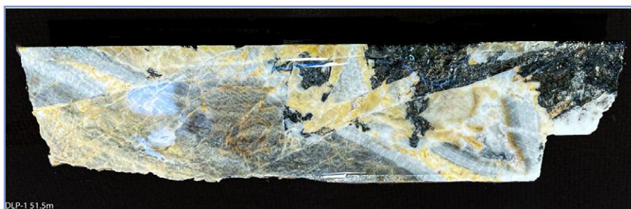
Figure 5 Example of coarse sphalerite infill (black) in BHP's diamond hole DLP-1 (51.5m depth).
