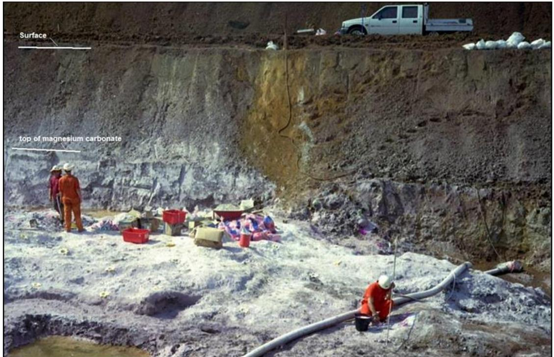
Figure 9 Test mining of magnesium at Winchester during the wet season (preparing to blast Level -1)
