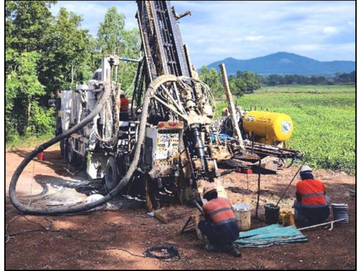
Left and above: Chang Phueak Prospect, RC drilling Hole #2
