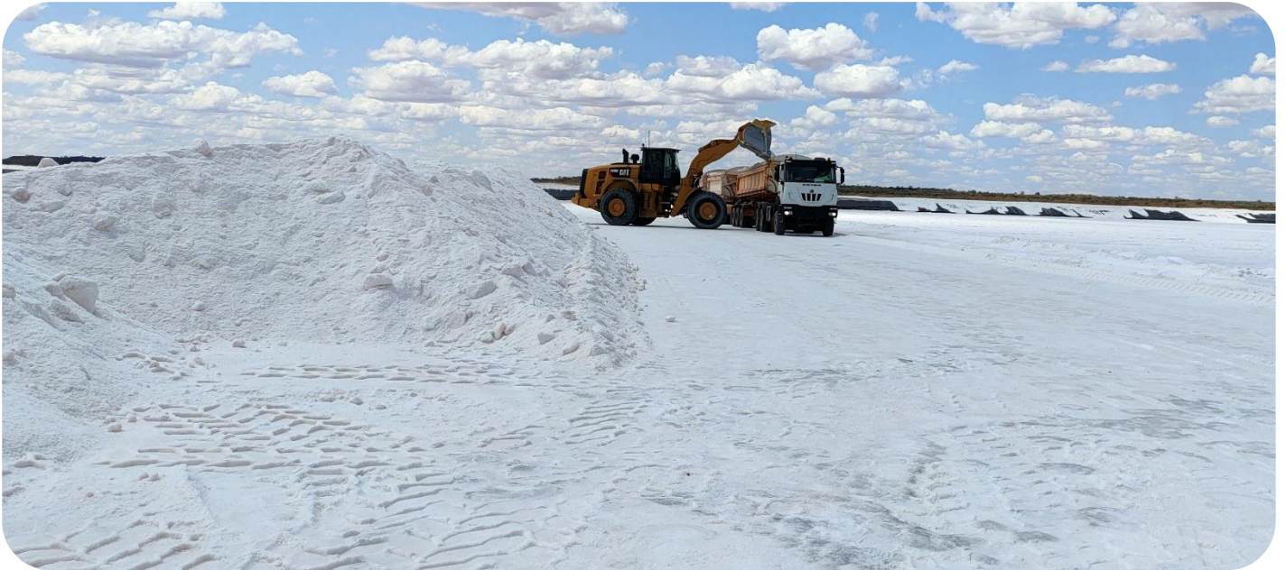
Alternate harvesting method trial using dozer (not pictured) and front end loader, September 2022
