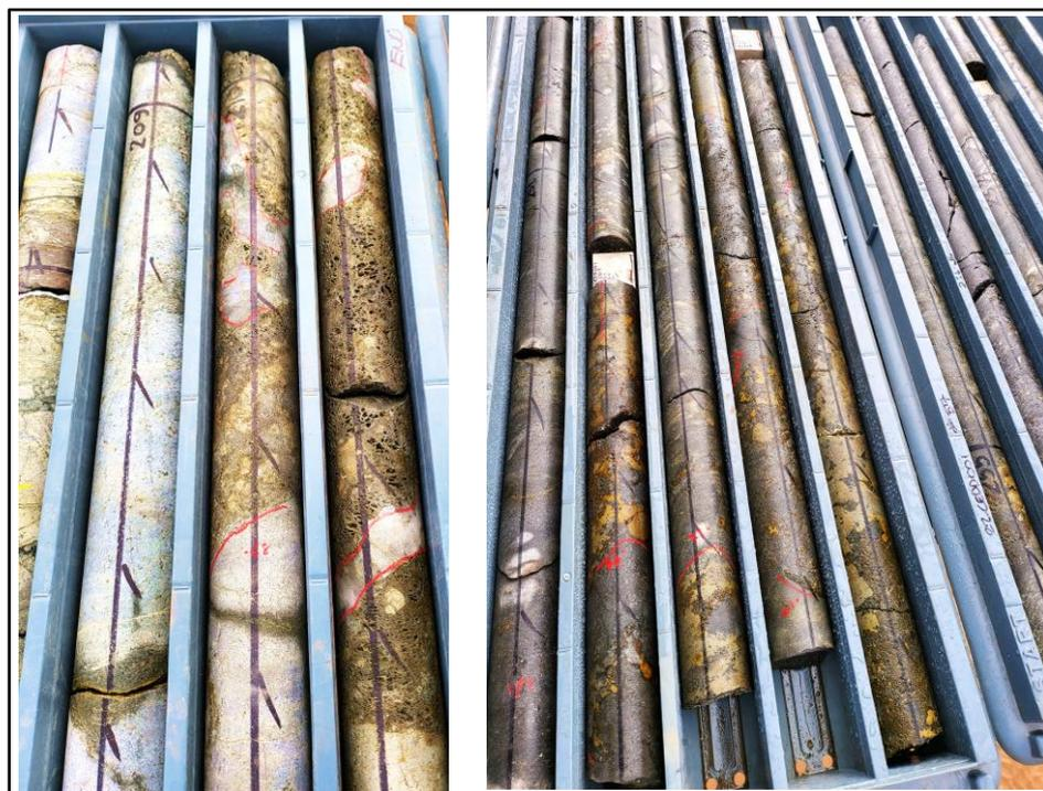
Figure 1: Massive sulphide 22CEDD001
