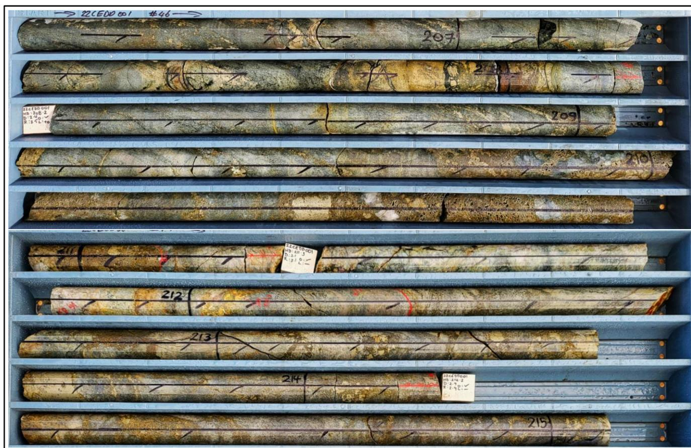
**Figure 3:** 22CEDD001 drill core 208.2m-215m, massive and highly disseminated sulphides
