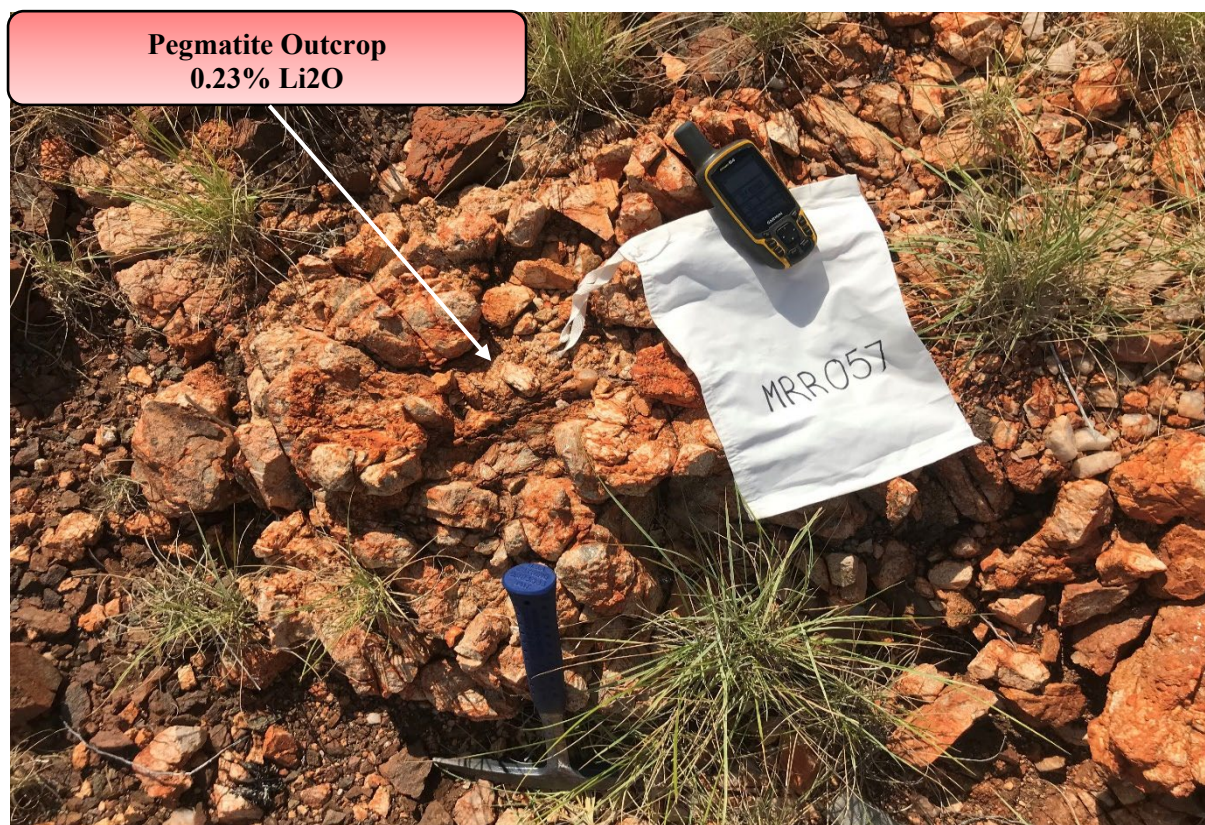
Figure 7 – Sisters (Southern Zone) pegmatite (Sample MRR057- 0.23% Li 2 O) Feldspar-quartz-mica-sericite pegmatite, near 130 ppm Li soil result
