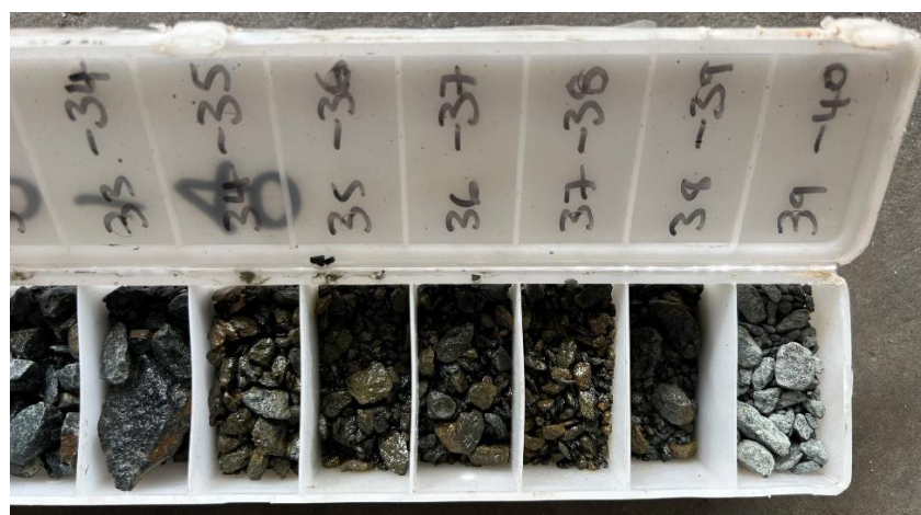
Figure 1. 4m of visible chalcopyrite from 34m to 39m in GRRC005.
