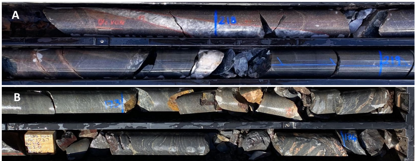
Figure 5. A, Core tray photograph of quartz-pyrite vein intercepted within sandstone at ~218m, TMDD0001. B, folded and sheared sediments (shale), with k-feldspar, silica and pyrite alteration, indicative of hydrothermal alteration at ~173m.
