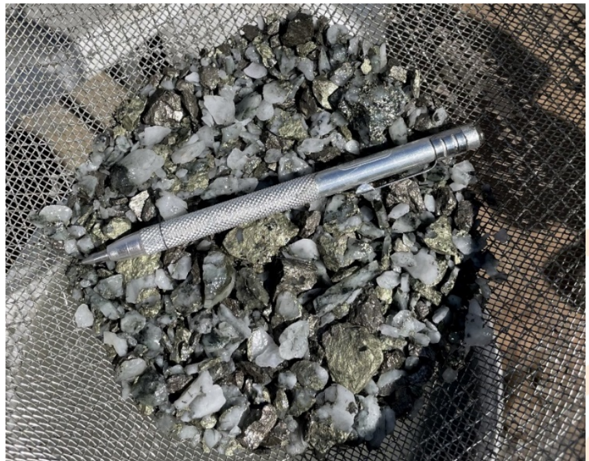
Figure 1. Sieve of sulphidic interval, 80-81m in HMHSRC001 which analysed 5.04% Cu by portable XRF
