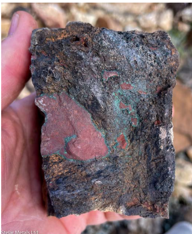
Figure 3: Left: View of the historical Line of Lode at Baratta Copper Mine, Right: Example of discarded copper ore on old working within the granted EL (XRF: 36% Cu and 478 g/t Ag)
