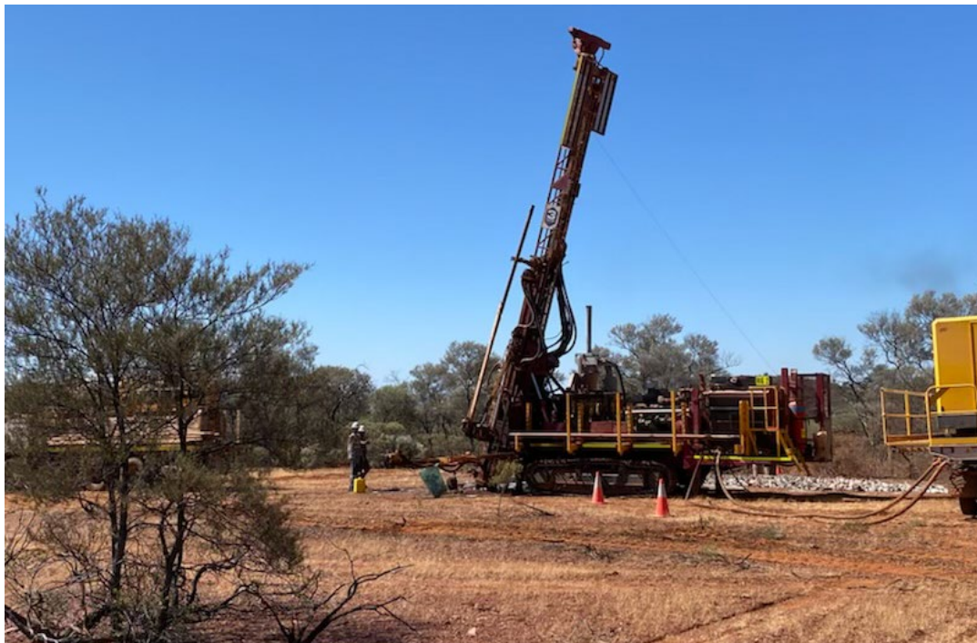
Image 1: RC Drilling underway at the Mount Boggola Project.
