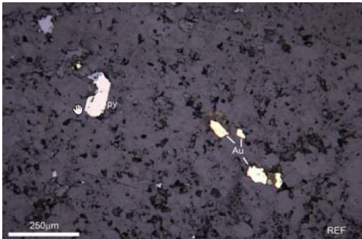
Figure 3: Mulgabbie North Demag Zone diamond core reflected light polished section MNODH 006 425-426m (0.32 g/t Au) free gold associated with pyrite
