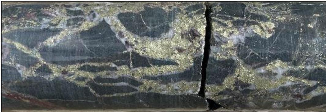
**Photo 1. Chalcopyrite-quartz-hematite fill jigsaw breccia in chlorite-silica altered microdiorite - SMD173, 390.6m drill depth, HQ diameter uncut drill core. Note the dominance of chalcopyrite and hematite and the almost total lack of pyrite as distinct from the previous samples in SMD032, SMD044W1 and SMD050.**
