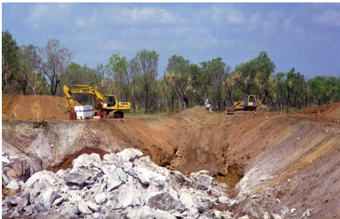
Figure 9 Test mining of magnesium at Winchester during the wet season (after blasting Level 0)
