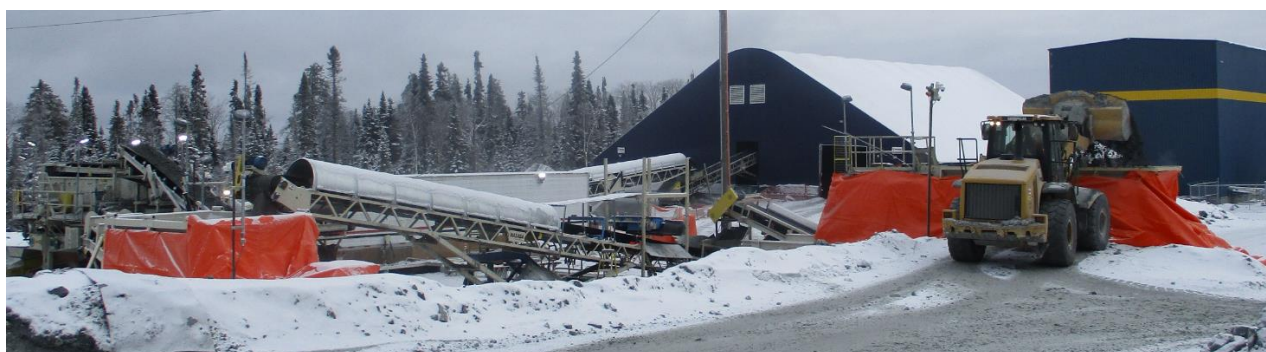
Figure 3: New Sugar Zone crushing circuit
