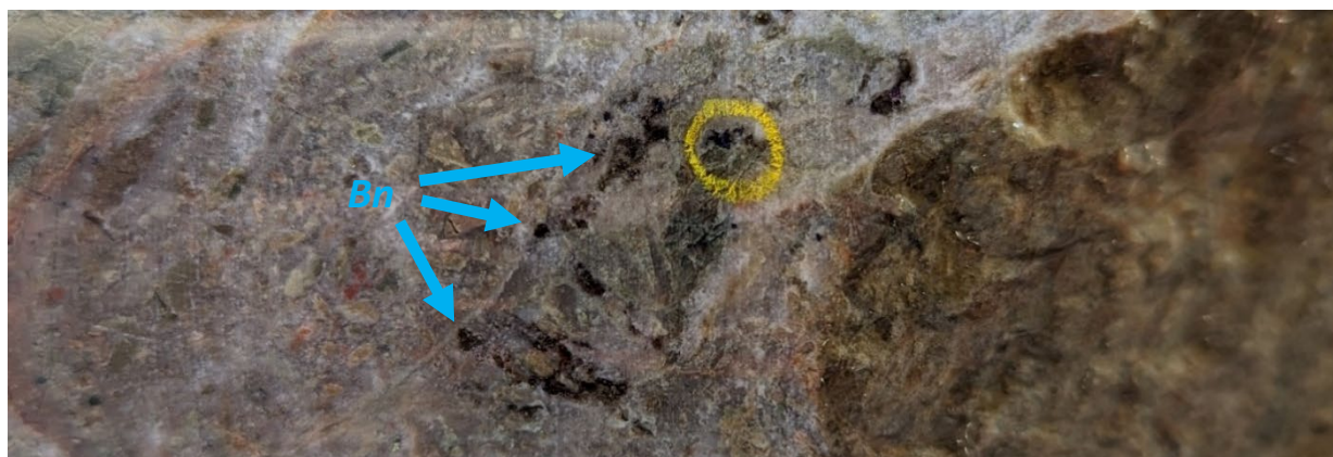
Figure 7 – Copper mineral bornite (dark blue) in chlorite-altered, quartz-veined metasedimentary rocks (577.4m),
