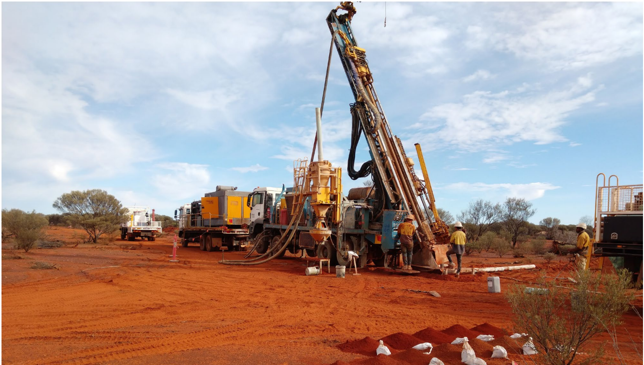
Figure 4: RC drilling at Indomitable
