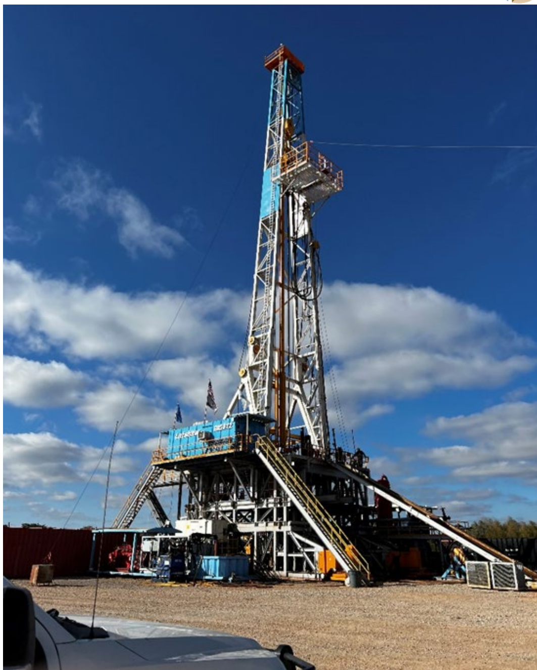
Figure 6. Latshaw Drilling Rig 12, drilling ahead on the Wolf Pack Well location, Stephens County, Oklahoma
