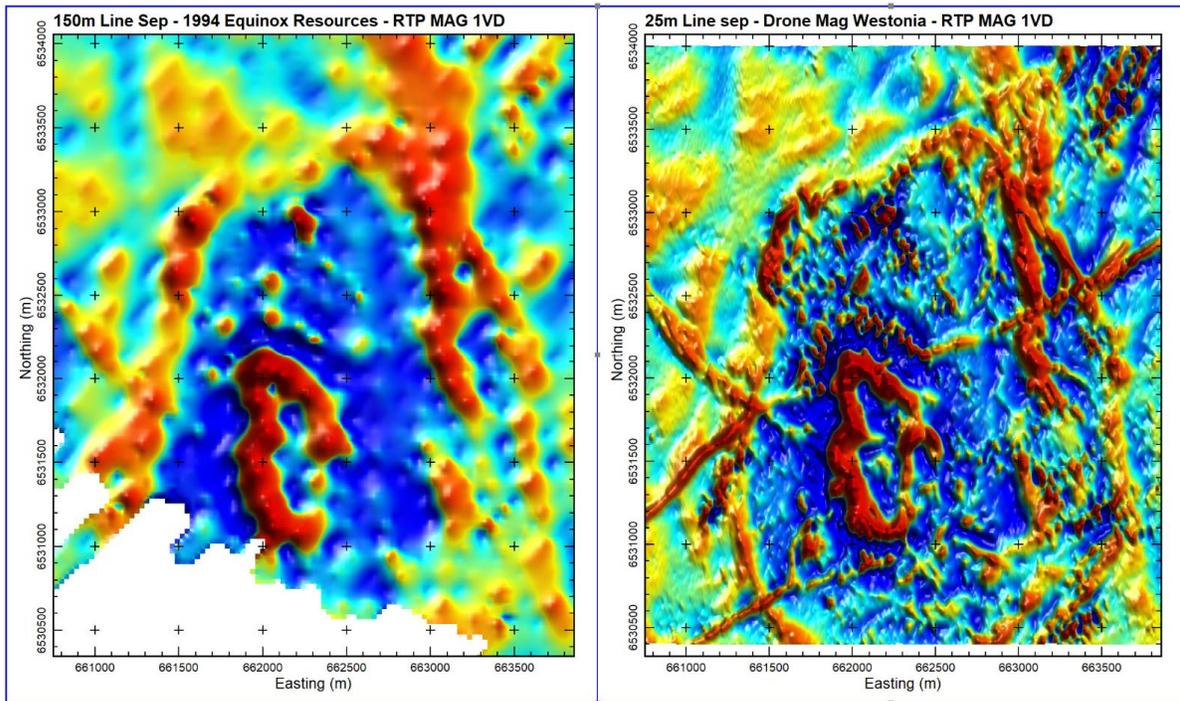
Figure 4: Drone magnetics 25m line spacing and 25m flight height providing an excellent high-resolution image of the Westonia eye (right image) over the previous 50m flight height and 150m line spacing regional public Magix version (left image).
