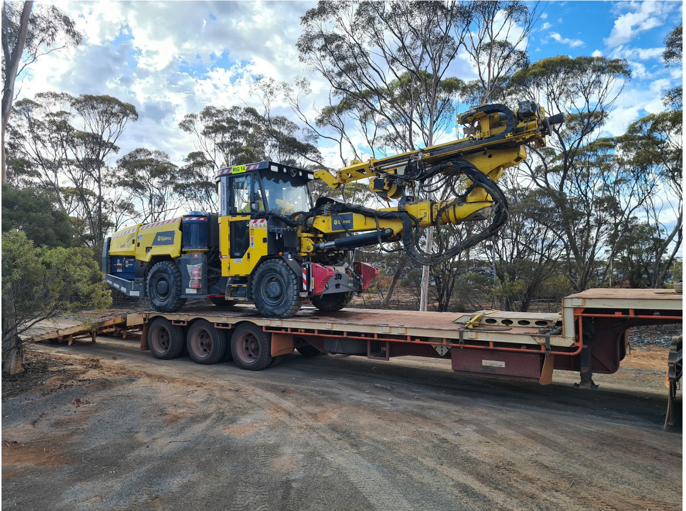
Figure 16. Underground diamond drill rig mobilised at Cassini.
