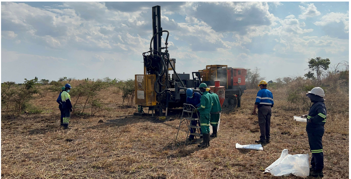
Figure 3: AC drill rig in action during the program
