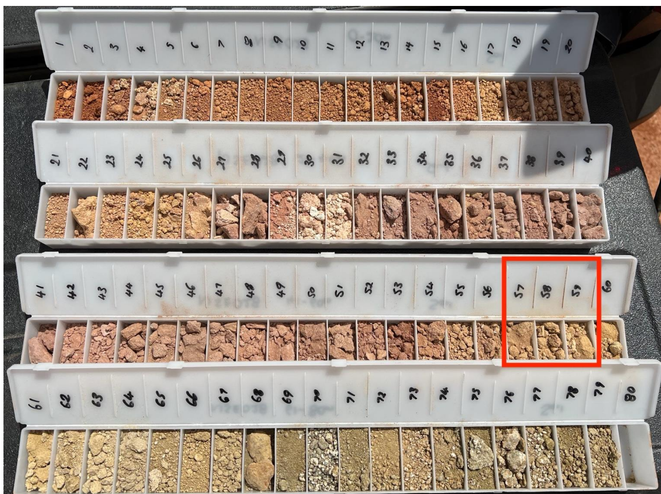
Figure 2. Air Core samples from NSE028 showing weathering variation REE enriched regolith at North Stanmore. Note the interval between 57-60m with 1.01% TREO highlighted in Red.
