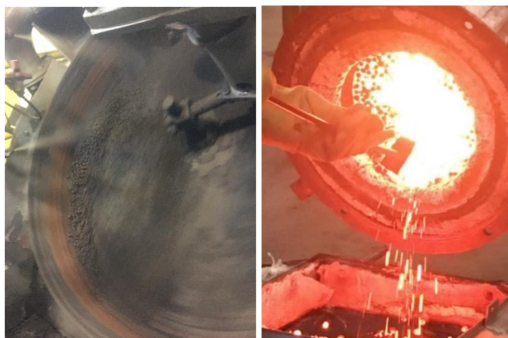
Figure 2 – Pilot process for pelletised roasting
