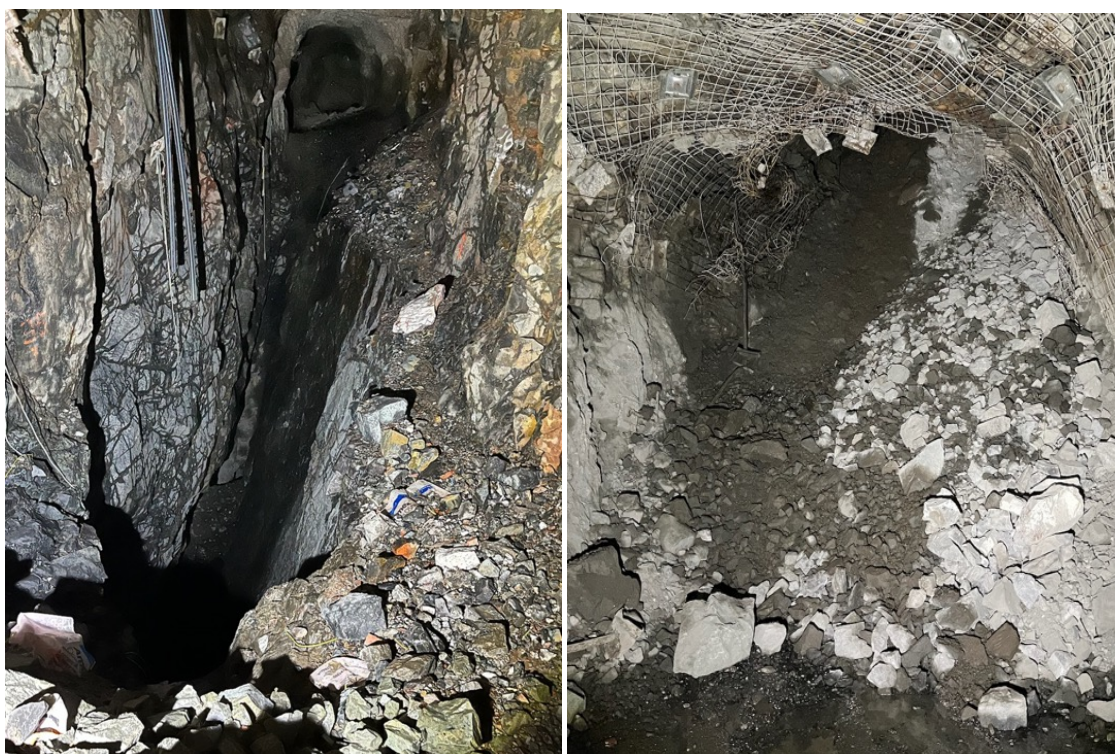
095 level stope void from above Stope ore reporting to 105E level
