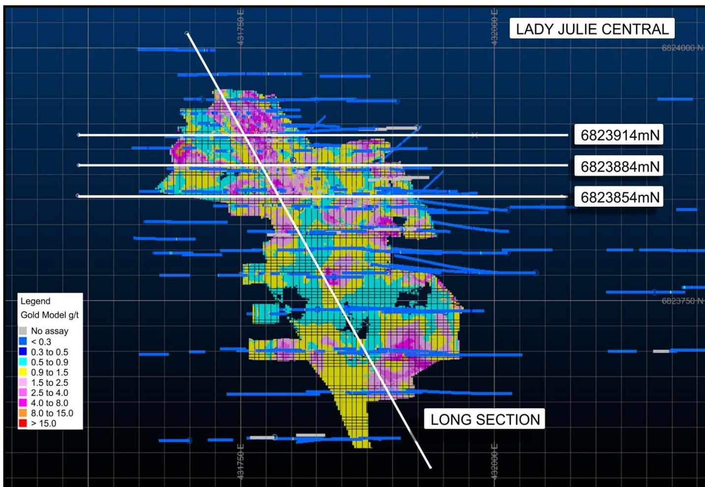
Figures 3 a), b), c). Lady Julie Central cross sections showing main gold intersections and resource wireframes and block grades.
