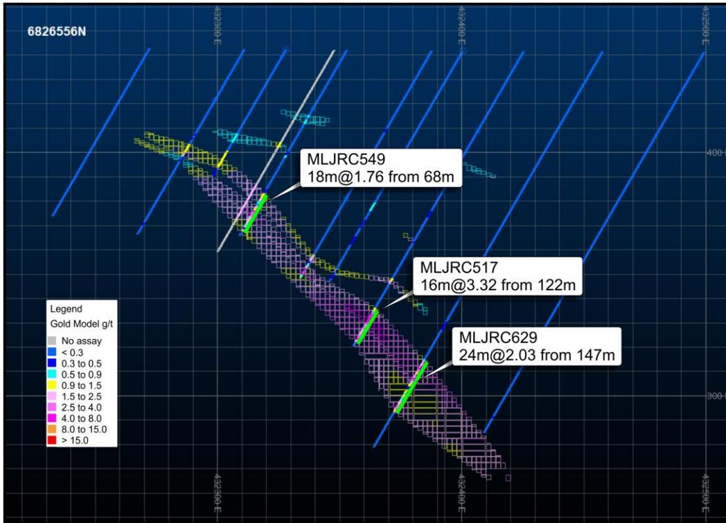
**Figures 7. Lady Julie North 4 Long Section showing main gold intersections, resource wireframes and block grades.**
