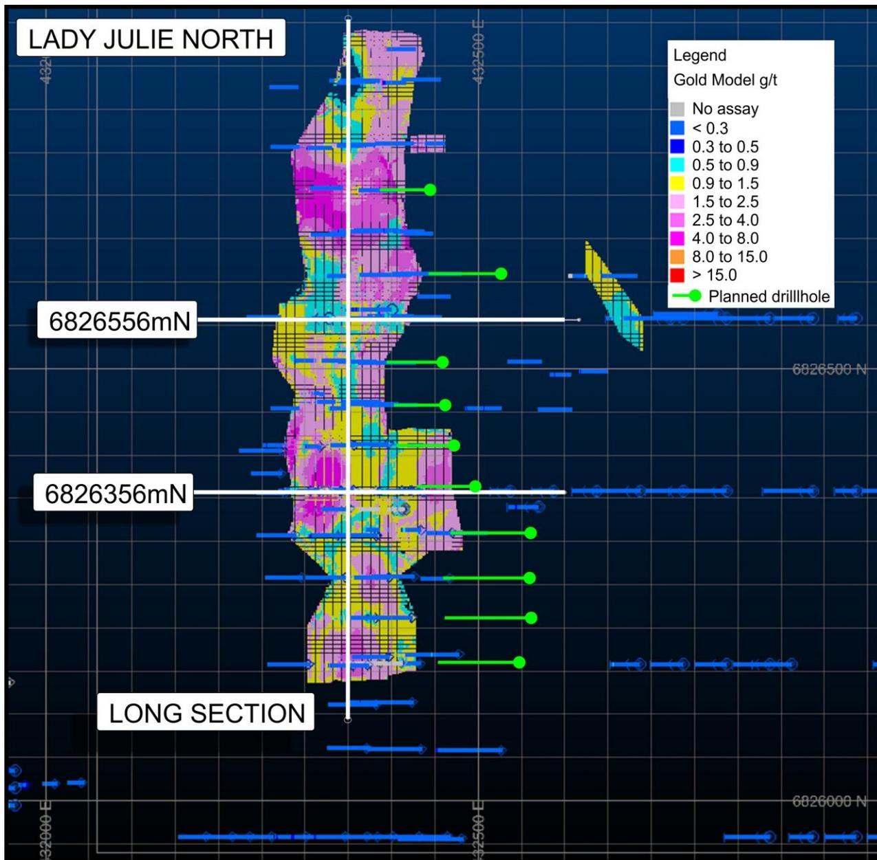
Figures 6 a) and b). Lady Julie North 4 cross sections showing main gold intersections, resource wireframes and block grades
