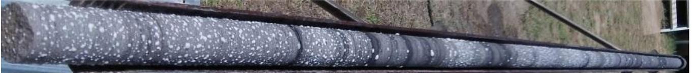
*Figure 3: 3m core sample from 475m showing gassy sandstone formations*
