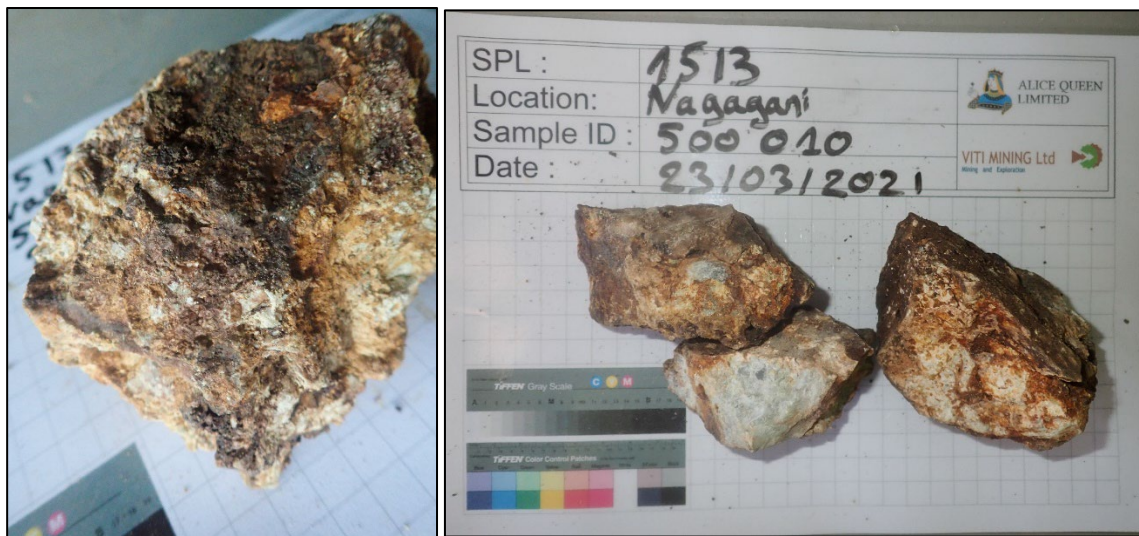
Figure 6. Weathered rock chip samples (alteration and vein) recently collected from the Nagagani and Karikarimasi creek area (Dakuniba Prospect, SPL1513) returning 4.6g/t Au (left) and 1.4 g/t Au (right) collected from an earlier reconnaissance trip.
