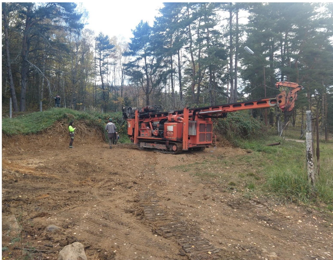
Figure 5: Diamond drill rig set up at the first target area, site preparation completed, location of drill hole SSD-01
