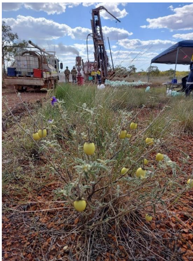
Figure 3. Tulla RC rig TD04 drilling BURC00686 to south of Anthill open pit.
