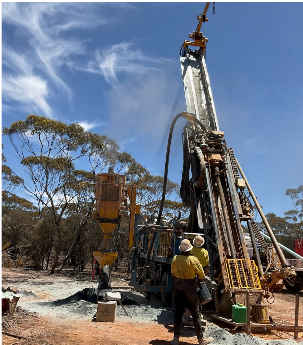
Image 1 – RC drilling at Hestia.
