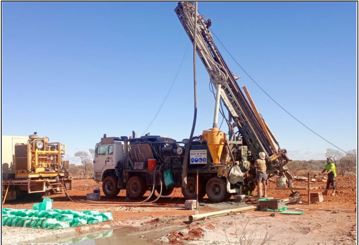
Image 2 / RC drill rig at Mt Eelya Cue/Murchison Copper Project, May 2022
