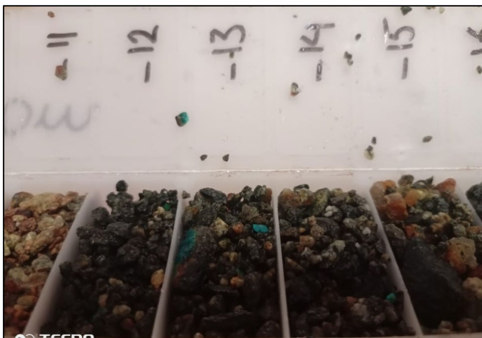
Image 3 / RC drill chips: 22CURC004 11m to 15m, 4m at 5,020 ppm Cu and 8,720 ppm Zn
