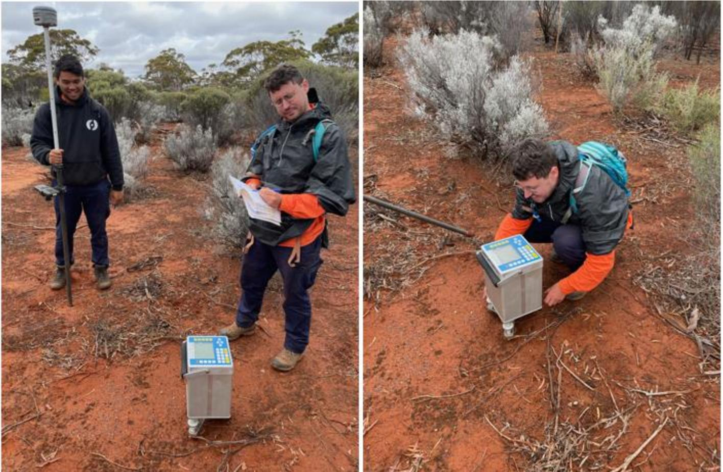
**Figure 2: Technicians taking gravity readings at Hickory.**
