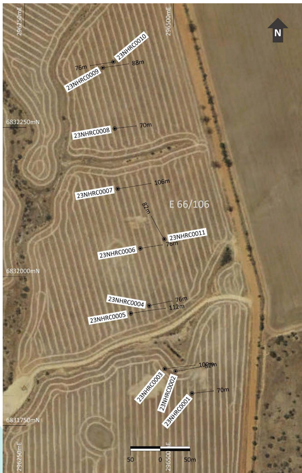
Figure 3: Lady Sampson completed RC collar plan with aerial image.
