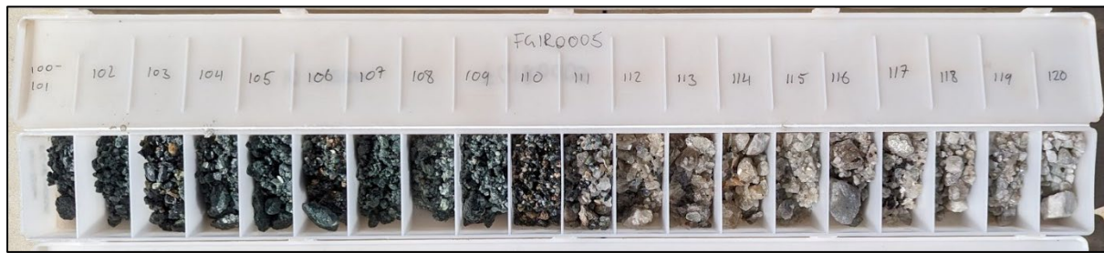
Figure 5: FGIR0005 chip trays showing 10m of pegmatite from 110m
