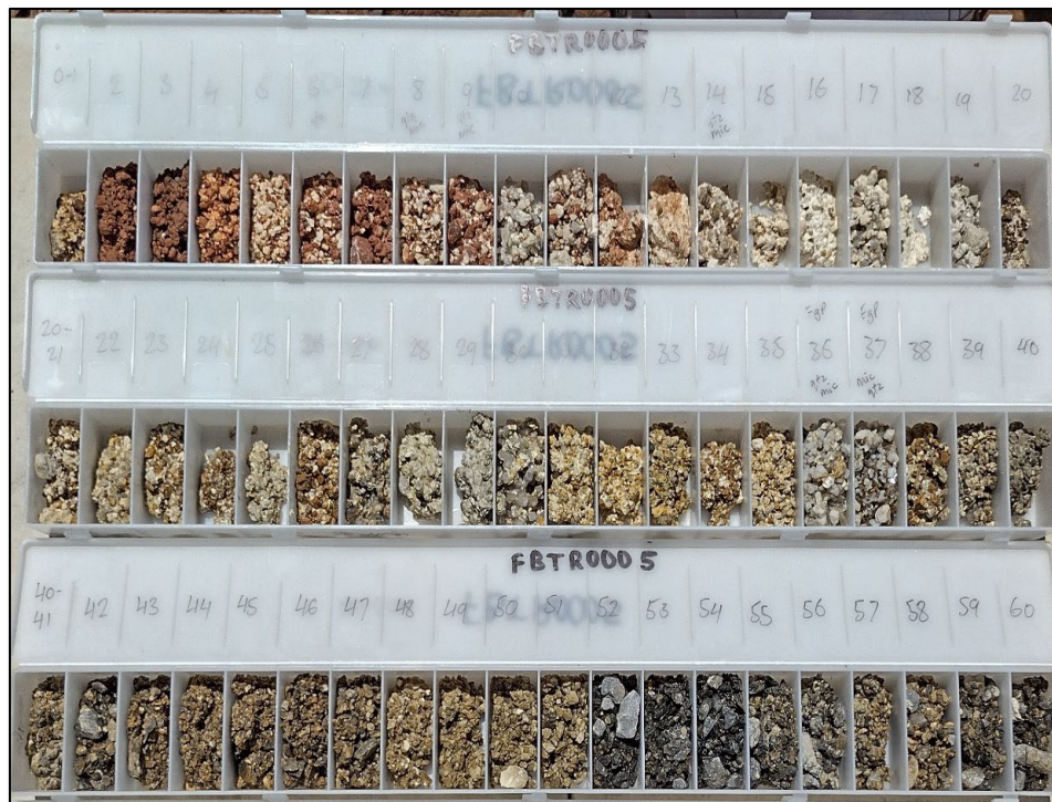
Figure 8: FBTR0005 where material from 7 – 21m was interpreted as highly weathered pegmatite with quartz, white clay and trace muscovite. Pegmatite also logged from 35 – 37m
