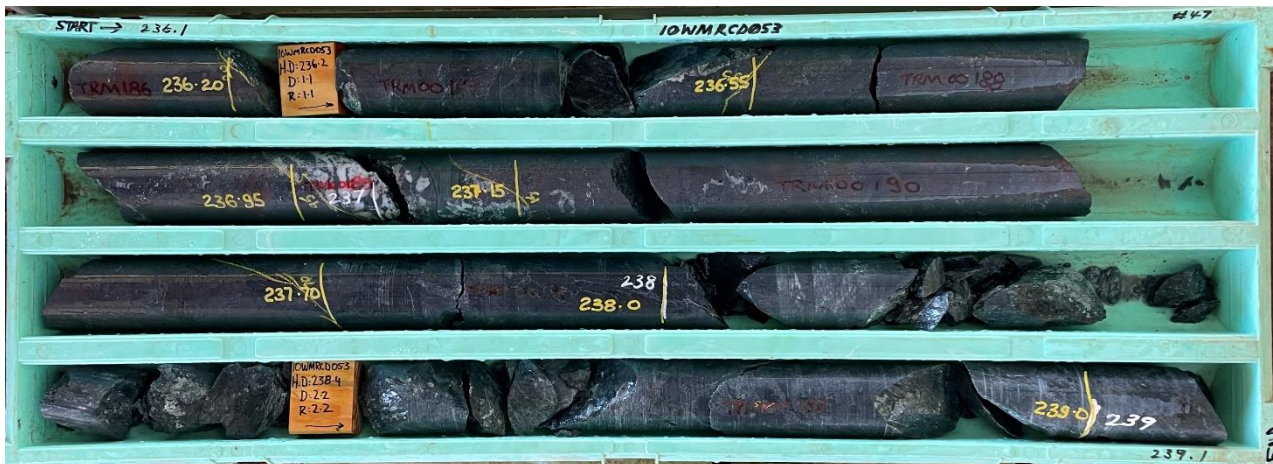
Figure Three: Massive Hematite Shale – Silicified – Minor lamination - (10WMRCD053)
