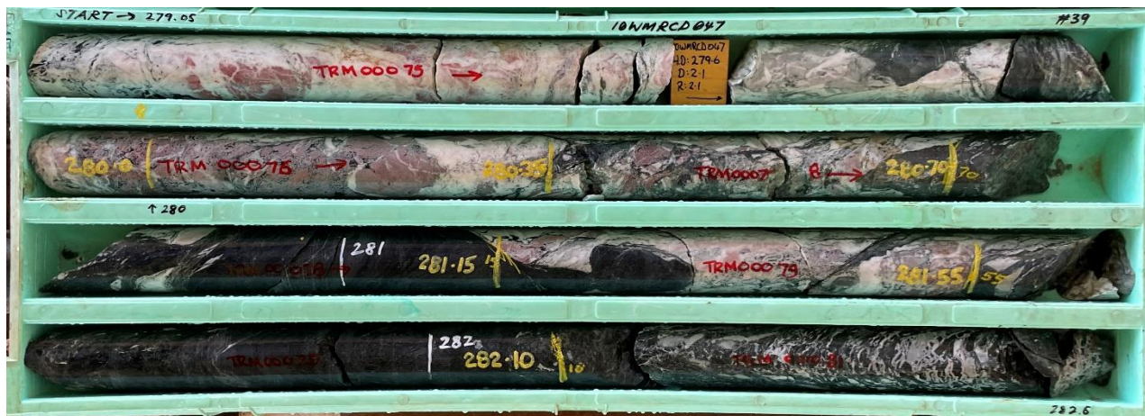
Figure Four: Transitions in Repeated Mineralisation Sequences – (10WMRCD047)
