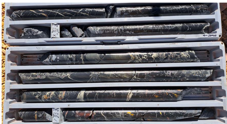
Figure 2. Diamond drill core containing sulphide copper mineralisation from drillhole MTKD010 at Flying Horse pit.
