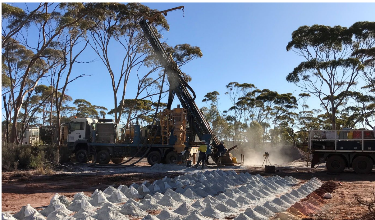
Image 1 – RC drilling Theia in-fill
