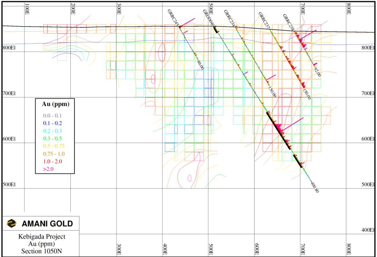
Figure 1 – Cross Section 1050N showing GRDD040 and the 2020 resource model blocks and Au (ppm).
