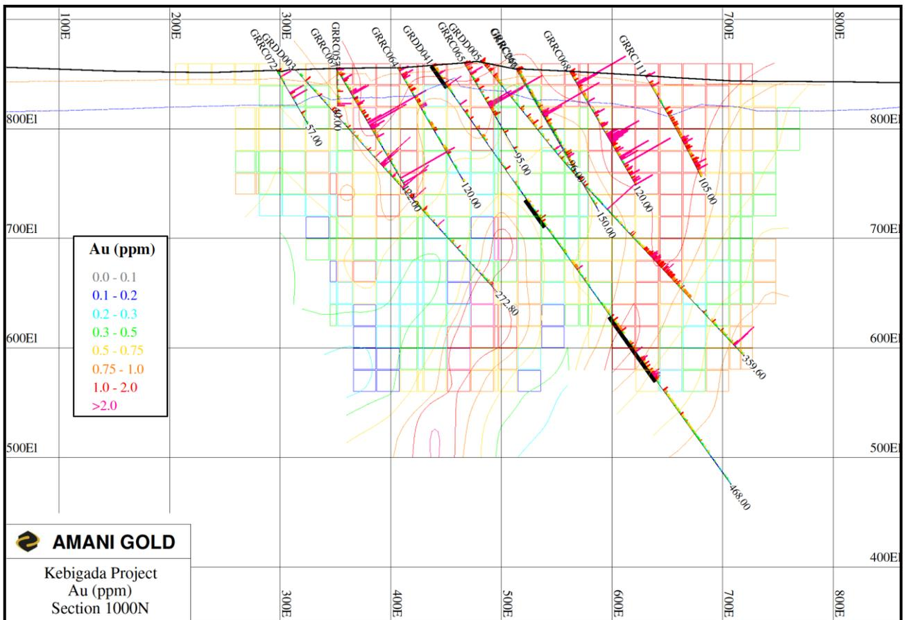
Figure 2 – Cross Section 1000N showing GRDD041 and the 2020 resource model blocks and Au (ppm).
