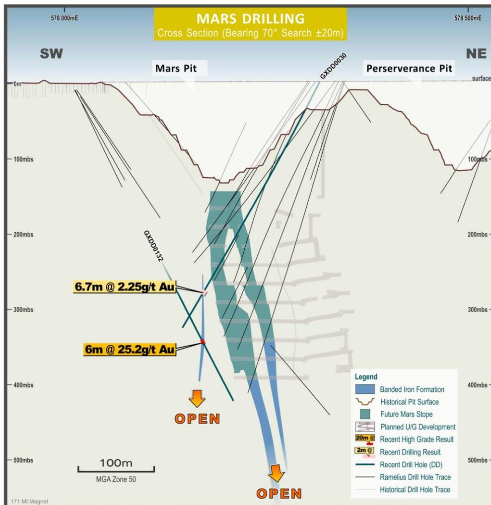
Figure 3: Mars - cross section with recent drilling results
