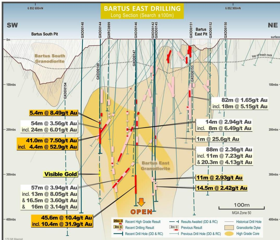
Figure 4: Bartus East – Long section with recent drilling results
