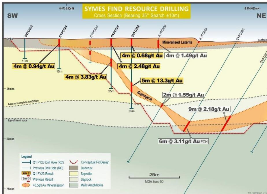
Figure 5: Symes Find cross section with concept pit design and recent drill results
