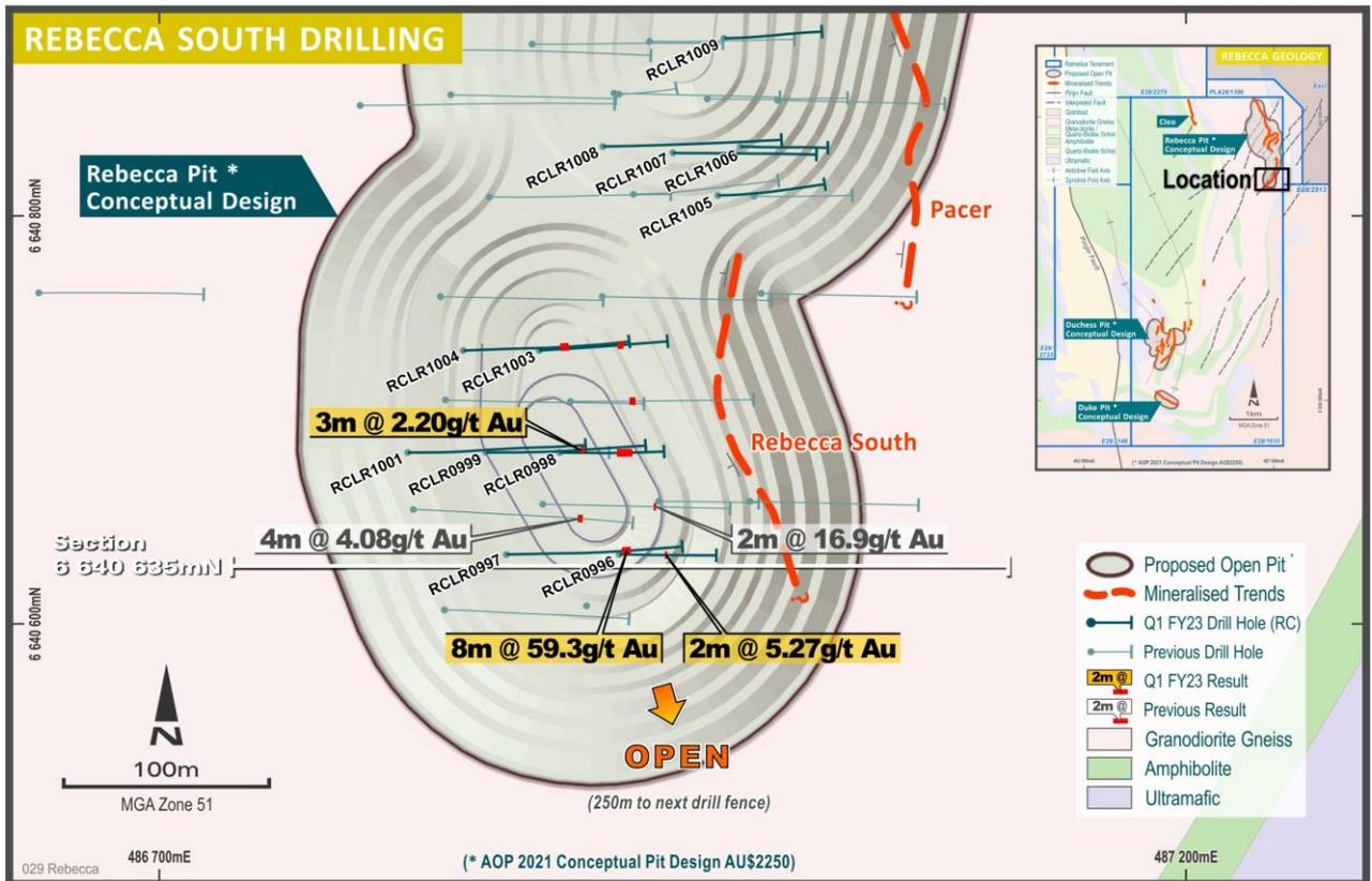
Figure 6: Rebecca plan view showing conceptual pit design and recent drill results
