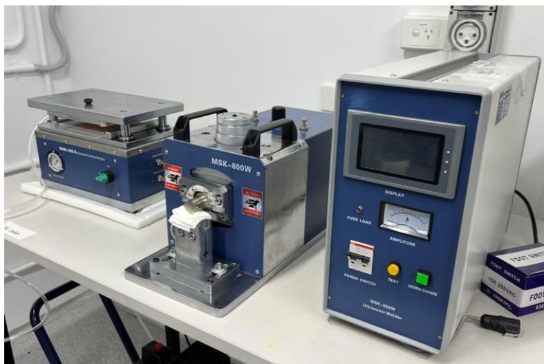
Figure 5 – Pouch Cell Assembly Equipment
