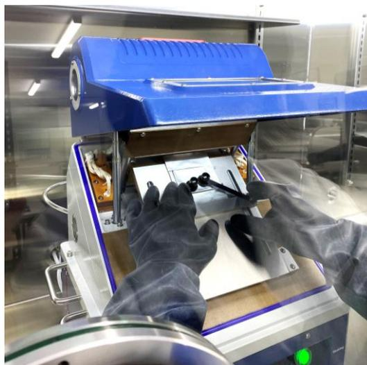
Figure 3 – Pouch Cell Vacuum Sealer
