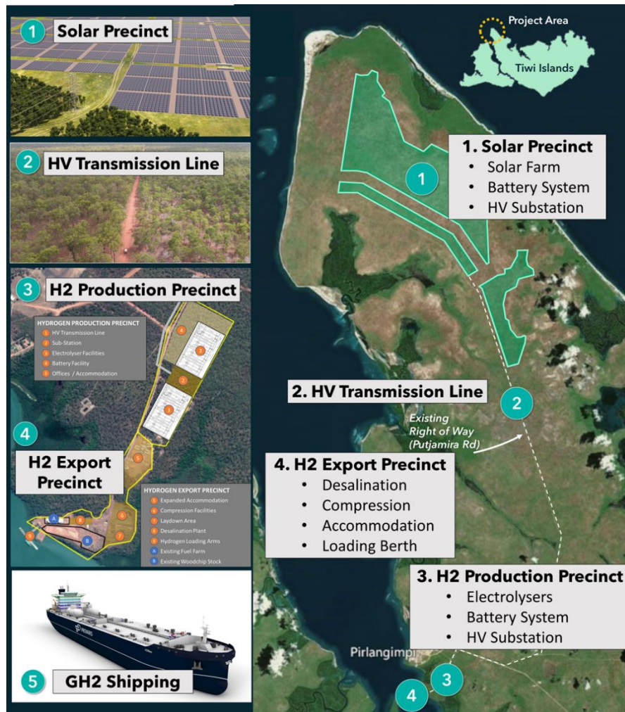
Figure 3: Illustration of Tiwi H2 Project proposal footprint and site layout.
