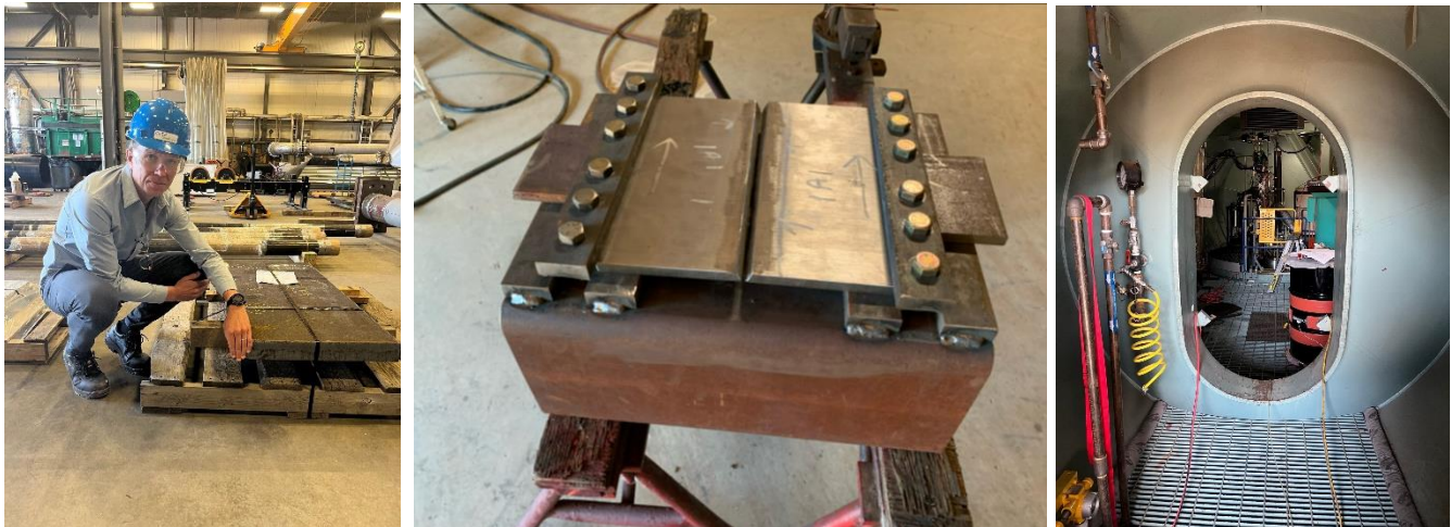
Figure 7: Provaris CTO, Per Roed, with sample structural plate. Plates prepared for welding. And photo of the special environments lab that will be utilized to test materials in a hydrogen environment.
