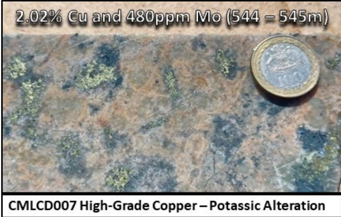
Figure 3: High-grade Cu mineralisation hosted within potassic alteration, CMLCD007.
