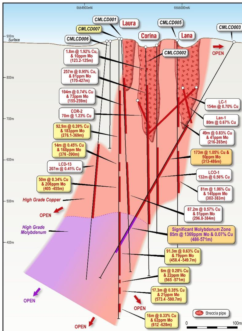
Figure 1: Long section (+/- 100m) looking north (section B-B') showing position of drillholes and targeted breccia units.
