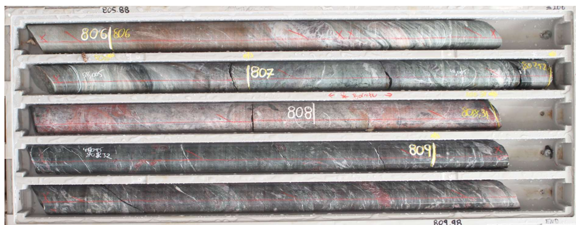
Figure 1. Drill core showing alteration and lithology logged around the trace/minor bornite mineralisation within exhalative sediments at 808m. Size of drill core = NQ or ~47.6mm.
