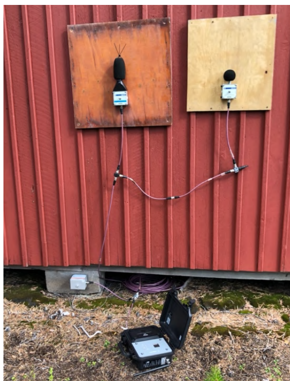
Figure 5 Trial mine impact monitoring includes dust (L) and noise (R) stations. These stations are collecting data as part of Talga's environmental management plan and commitment to environmental stewardship.
