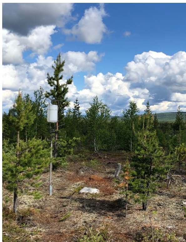
Figure 5 Trial mine impact monitoring includes dust (L) and noise (R) stations. These stations are collecting data as part of Talga's environmental management plan and commitment to environmental stewardship.
