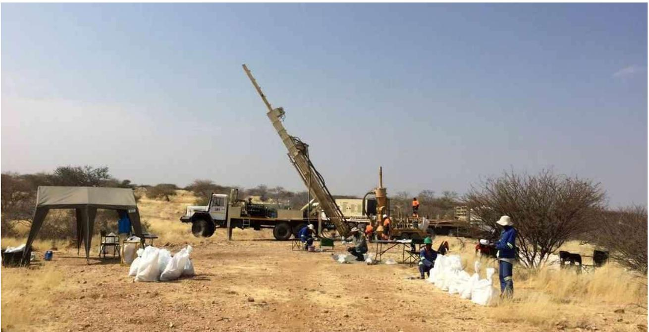
*Figure 4 – RC drill rig at Kokoseb*
