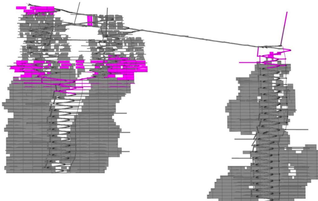
Figure 6: Sugar Zone long section showing FY23 mine schedule (magenta) v LOM design
