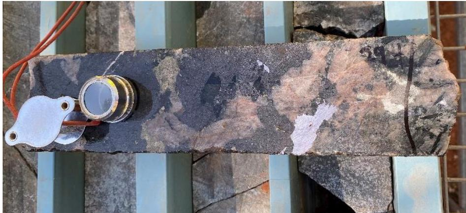
**Photo 2:** 21MHDD002: 293-294m (293.8m) - 1m @ 0.03% WO<sub>3</sub>, 0.04% Mo and 0.06% Cu – significant visible molybdenite and chalcopyrite visible throughout intercept, contrasting to assays
