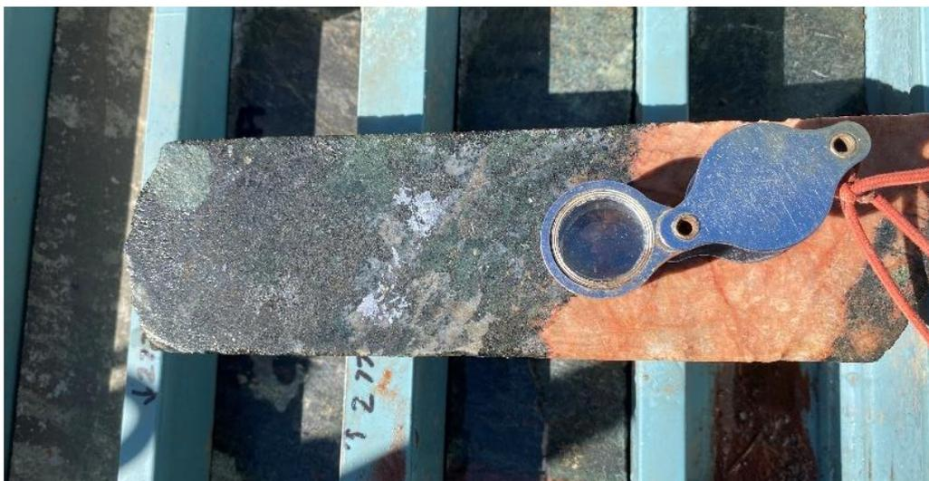
**Photo 1:** 21MHDD02- 282-283m (282.4m) - 1m @ 0.02% WO<sub>3</sub>, 0.23% Mo & 0.07% Cu - coarse grained visible molybdenite in magnetite skarn
