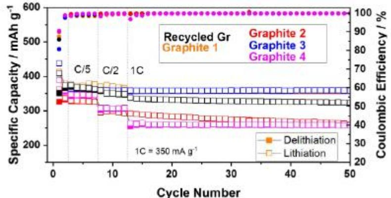
Electrode contains: **95% recycled graphite** (+3% SBR, 1% CMC, 1% C45)
