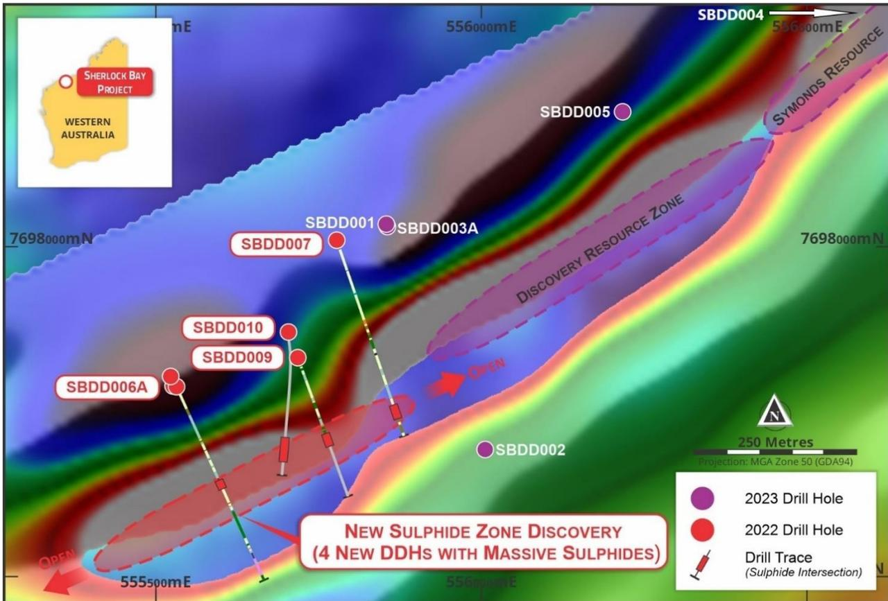
**Figure 3: Diamond drilling at Sherlock Bay which intersected the new sulphide zone with strong EM conductors.**
