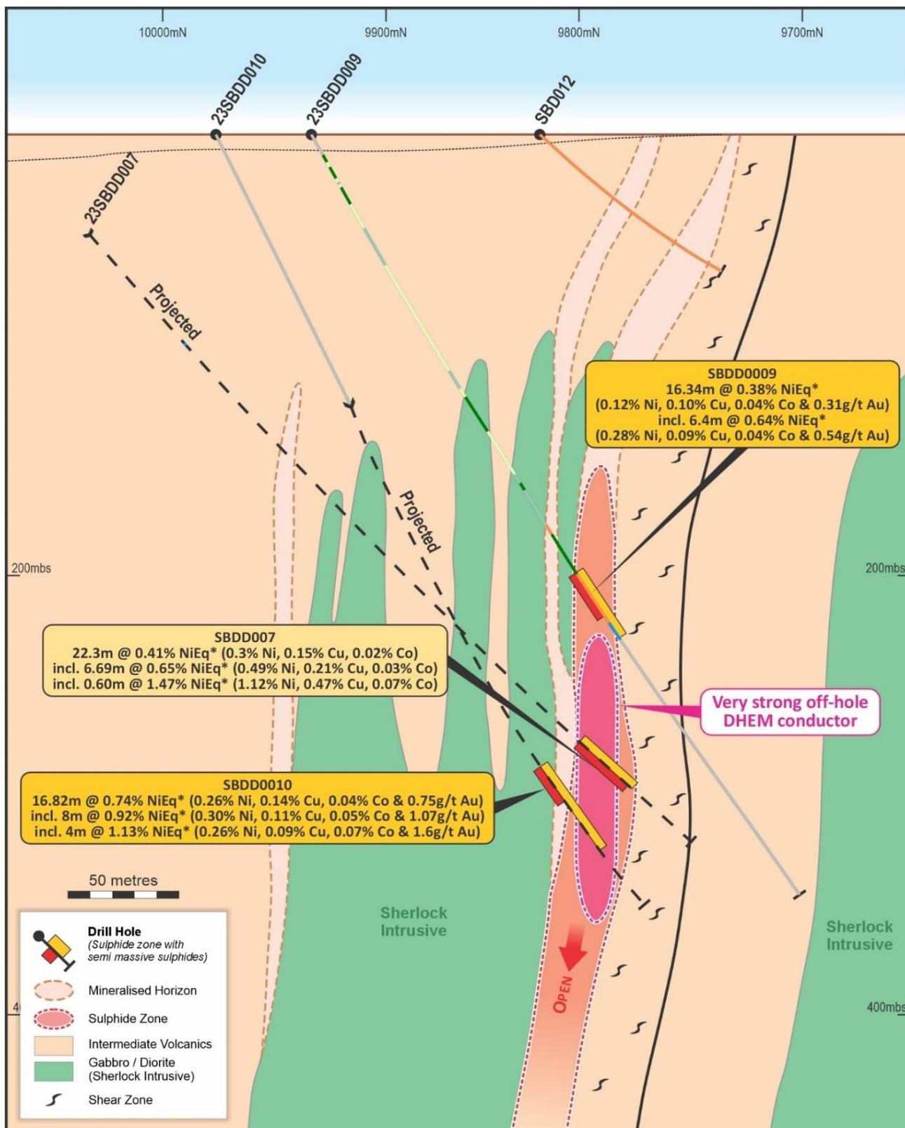
**Figure 4: Cross section 19,400mE showing significant sulphide intersections on footwall of Sherlock Intrusive.**
