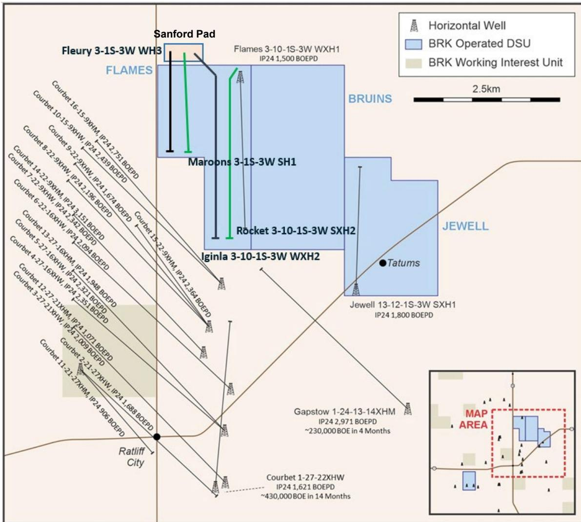
Figure 2: Location of the Sanford Pad and the four FMDP wells: Flcury, Maroons, and Iginla Wells (to be drilled from the Sanford Pad), and the Rocket Well (to be drilled from the existing Flames Well pad). Also shown are Continental Resources Courbet Wells full field development showing the strong performance of both the Woodford wells (well names ending with HXW) and Sycamore wells (well names ending in HXM).
